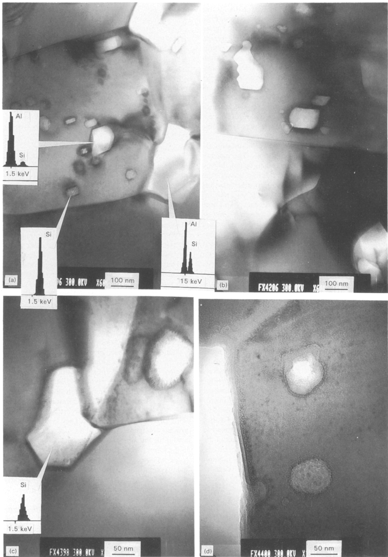
Figure 8 (a–d) Bright-field transmission electron micrographs showing the microstructure of the surface scale just behind the oxidation front in the nanocomposite aged at 1400 °C for 26 h. Both amorphous silica and aluminosilicate pockets were found to occur at the grain junctions and within alumina grains.
