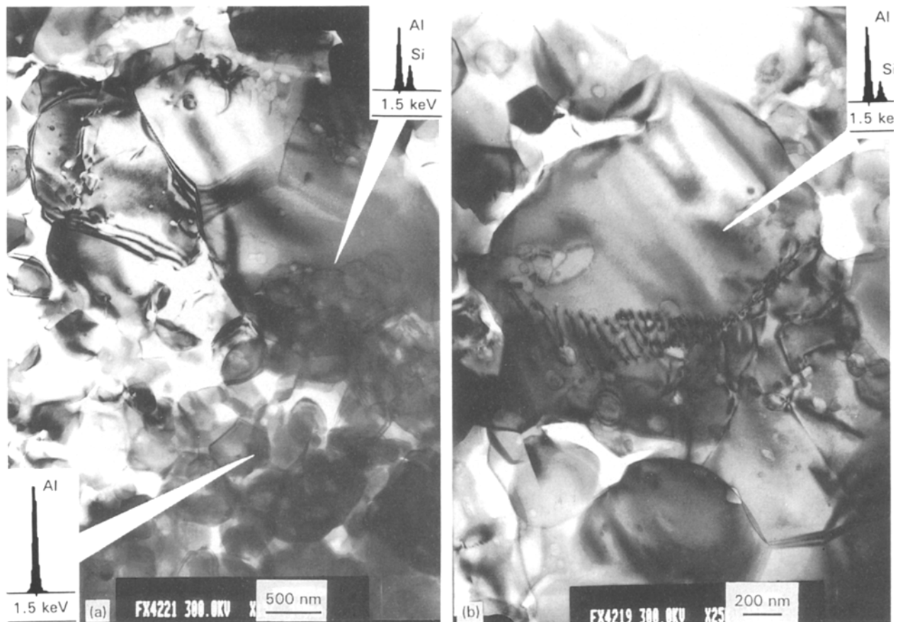
Figure 9 (a, b) Bright-field transmission electron micrographs showing the microstructure of surface scale approximately 30 \mu\text{m} from the oxidation front in the nanocomposite aged at 1400 ^{\circ}\text{C} for 90 h.
